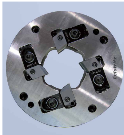
Tangential whirling tool for machining hydraulic-steering worms
