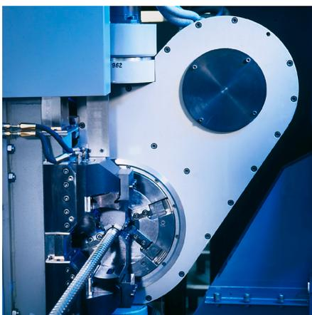
*Whirling tool with centering clamping rests in working position*
