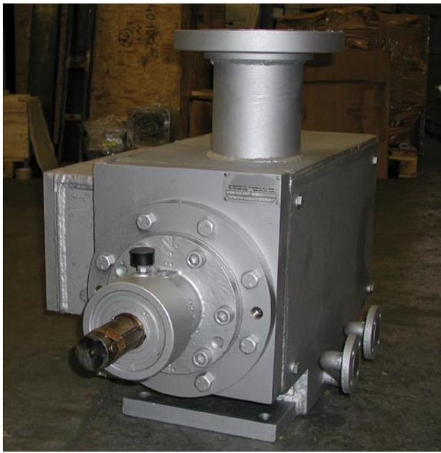
**This three screw asphalt transfer/loading pump replaced a timed screw pump at a refinery.**
