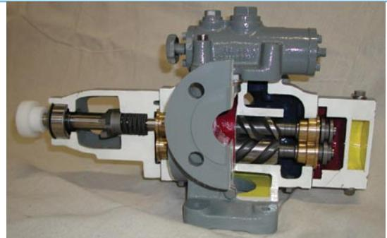
A cutaway model of a non-timed twin screw pump.
