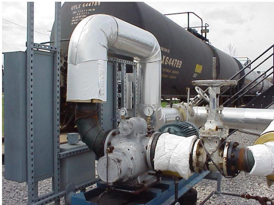
A non-timed twin screw pump for railcar unloading service at an asphalt terminal.
