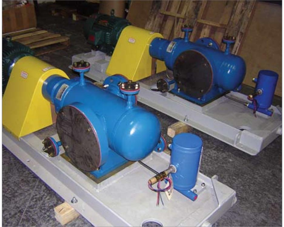
Leistritz screw pumps are hydraulically balanced and move liquid from suction to discharge as if it were being pumped by a piston with an infinite stroke. The low pulsation characteristics of screw pumps also eliminate the need for pulsation dampeners.
