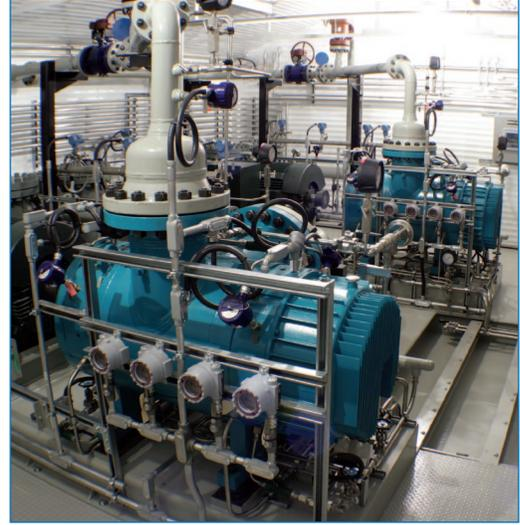
The Leistritz Multiphase Gathering System (MGSs) are expandable versions of the MWS, designed to handle production from multiple wells. Individual MGSs handle total flow rates up to 550,000 bpde
