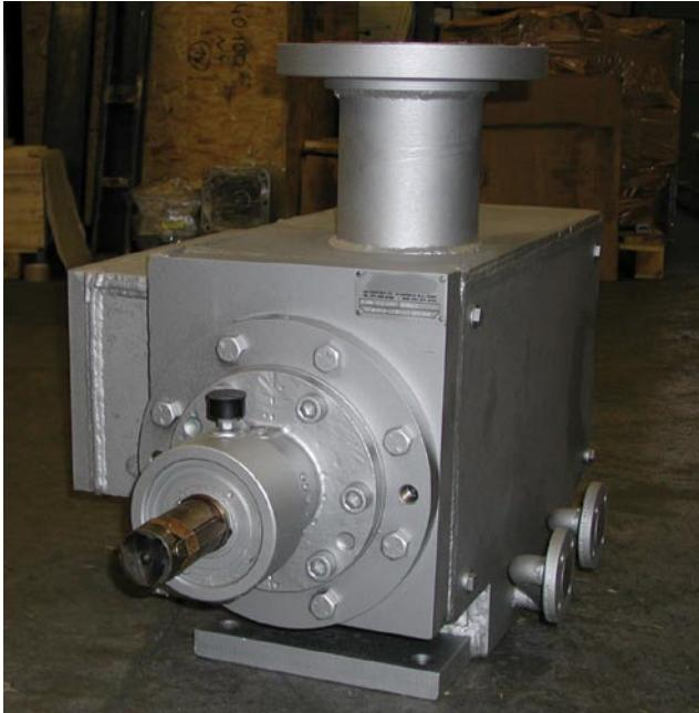
**This three screw asphalt transfer/loading pump replaced a timed screw pump at a refinery.**
