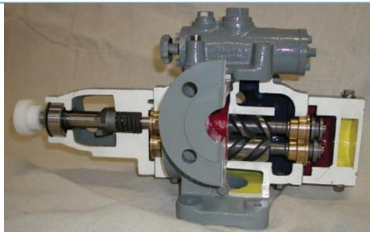
**A cutaway model of a non-timed twin screw pump.**
