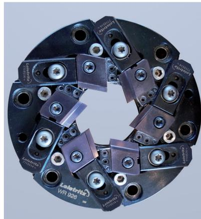
Tangential whirling tool for machining EPS-worms
