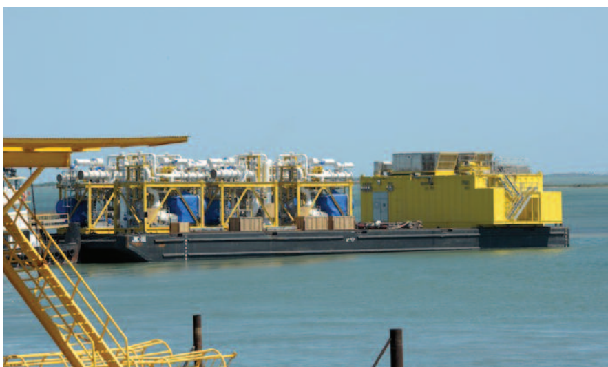
Shown here is a complete system delivery for an offshore platform. One of the advantages of installing multiphase pumps topside is a reduced footprint and eliminating vessels, tanks, pumps, compressors and other production equipment.
